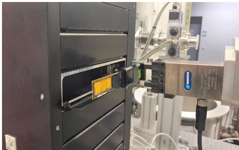
Figure 3: Gripper tool moving sample from the room temperature storage container
